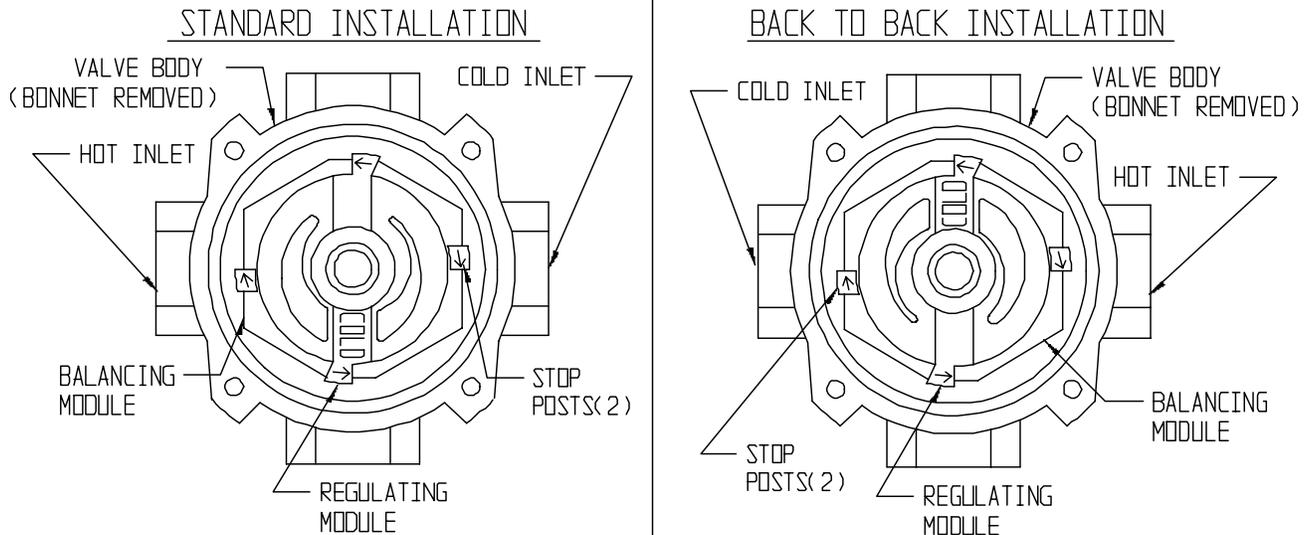
INSTRUCTIONS: PER THE INSTALLATION, POSITION REGULATING MODULE ON TOP OF BALANCING MODULE AS SHOWN. ROTATE REGULATING MODULE COUNTER CLOCKWISE UNTIL IT CONTACTS THE BALANCING MODULE STOP POSTS ("OFF" POSITION).
