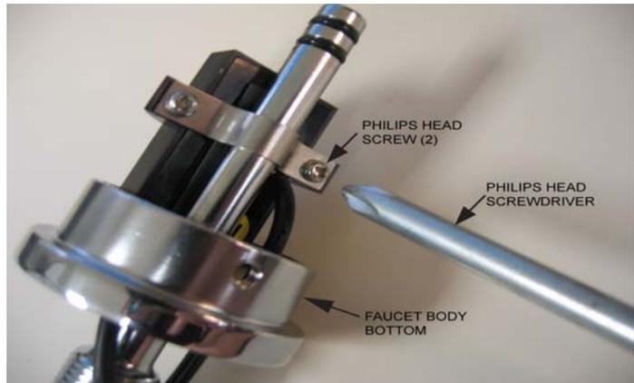
Reassemble new Module with care not to cut wires through the big holes into the Base, then insert the clamp with the Sensor over the shank. Tighten the 2 screws on clamp, making sure that the sensor sits on the flat of shank and touches the bottom of base. Grease the 2 O-Rings or change them if they are damaged. Take care when inserting Faucet Spout over the Sensor O-Ring and tighten the screw that was removed in the back.
