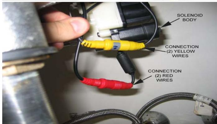
If the option has an UCM (under counter mixer), connect it to the inlet of the solenoid: -first by hand and then using an adjustable wrench (do not overtighten). **DRY CONNECTION ONLY.**
