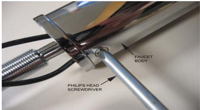
After screw has been removed from the unit, pull up faucet body top. There are 2 O-Rings on the shank and one around the lenses of Sensor Module that should be replaced if damaged.
