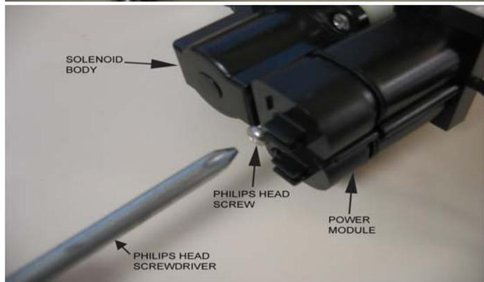
With the cover of the power module removed, remove the dead batteries and replace them with new batteries (ensure that the position of the new batteries matches the marks + and - on the cover). Replace the cover on Power Module.
